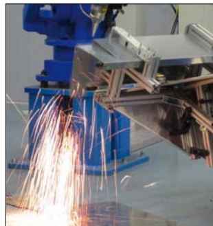
Components are manufactured using laser technology
