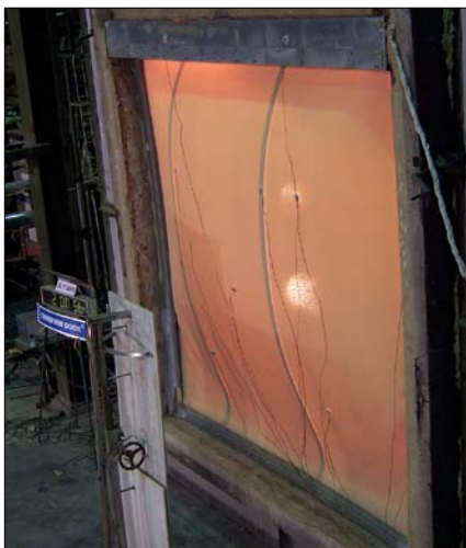
Testing a fire door at a research centre
